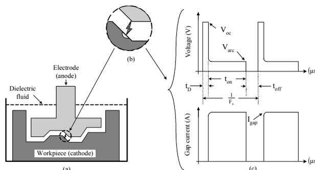
Figure 1. EDM Process
